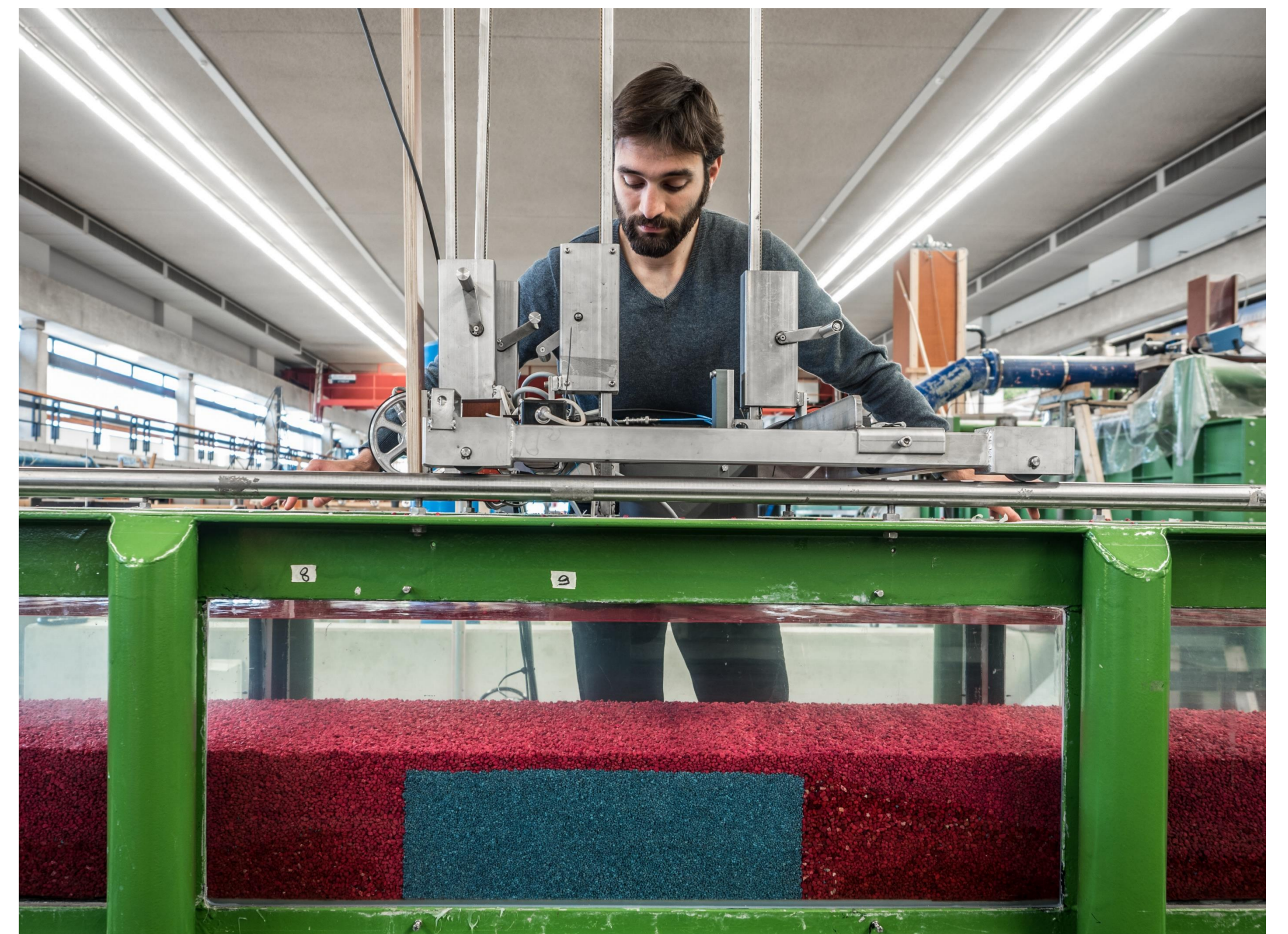
Laboratory experiments. We used two sediment size fractions: fine (blue) and coarse (red). Degradational conditions were imposed, causing the entrainment of fine sediment. The current model cannot predict this situation.
