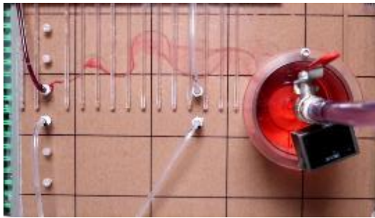
(1a) top view of small scale piping experiment
