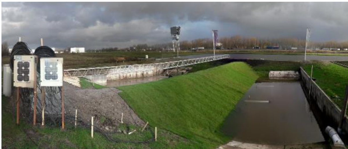
(2) Large scale piping experiment in Flood Proof Holland
