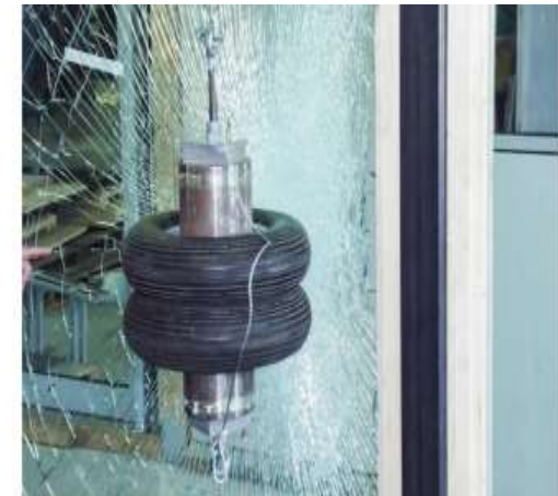
Figure 10-1: Pendulum test EN 12600 [GIB GMBH. (n.d.)]
