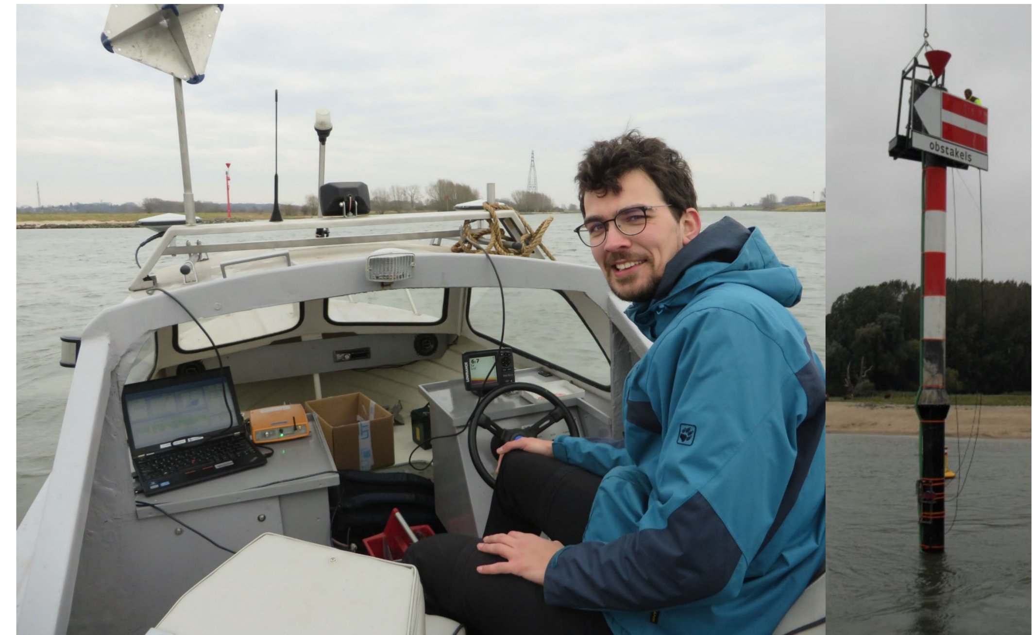
Flow velocity measurements performed with both vertical ADCP (left, spatial coverage) and horizontal ADCP (right, temporal coverage).
