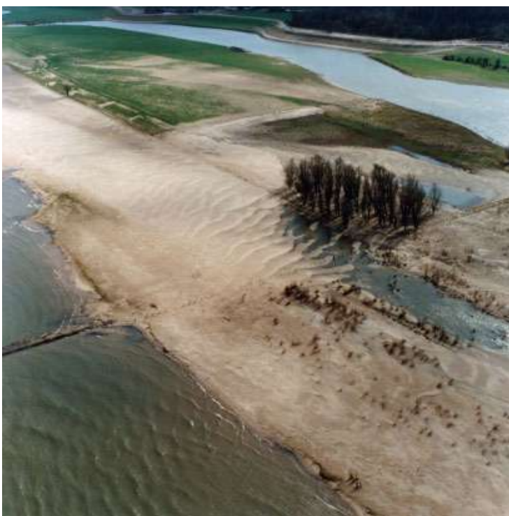
Theme 'morphodynamics during floods': sand deposition at the left bank of the Ewijksche plaat in the River Waal after the flood of 1995.
