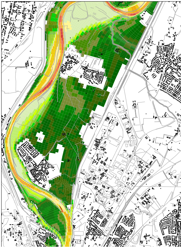
Figure 4. Results of WAQUA flow simulations: the village Borgharen is safe.
