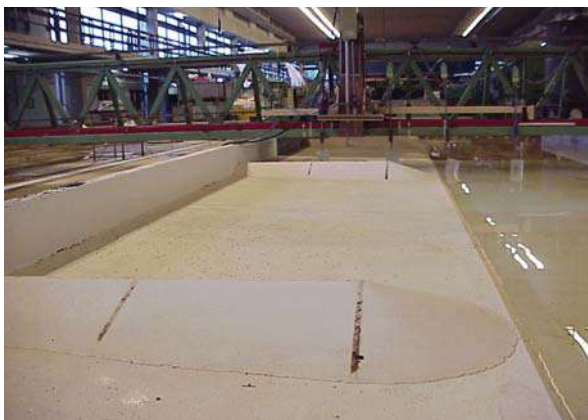
Figure 1. Physical model scale (1:40) to test effects of groyne design on water velocity at various water levels.
