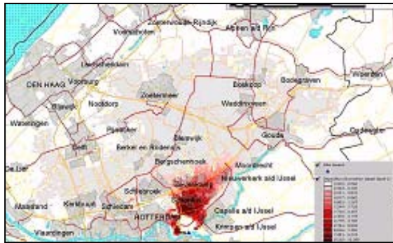
Figure 1. Deposition of sediment during the inundation stage, according to the ERA model [ \text{kg/m}^2 ].
