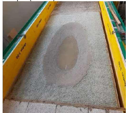
Figure 1. Experimental setup with a predefined scour hole in a fixed bed.
