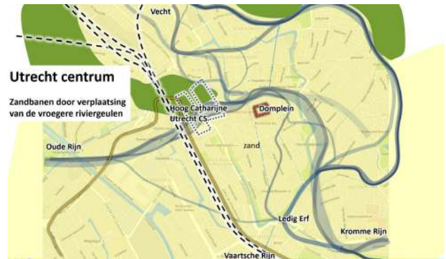
Figure 1. Roman and Medieval Utrecht Rhine and Vecht meanders (blue) and the sandy deposits (yellow) their migration left below most of the city.
