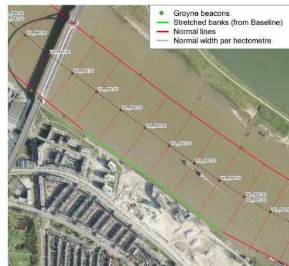
Figure 2. Resulting normal width along the Waal River
